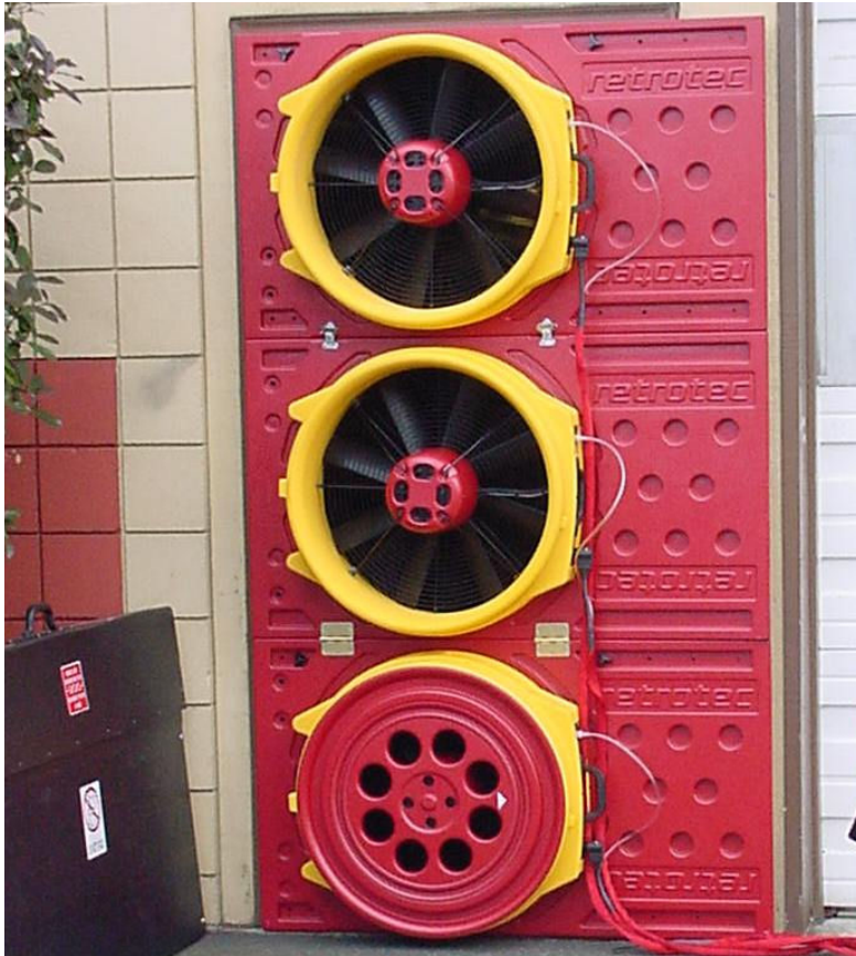
Retrotec Model QMG consists of one DM-2A, one DM-2, three 3200 Fans and a Light weight hard door panel for 3 fans. Add fan cases, software, grill mask and accessory options.
